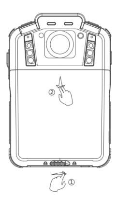
**Step1:** Drag the battery lock from the left side to the right side, and then the cover will be unlock. And keep the lock on the right side, and then go to step 2.
